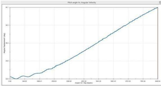
Figure 3. Graph between Pitch Angle of Blade & angular speed of Turbine
