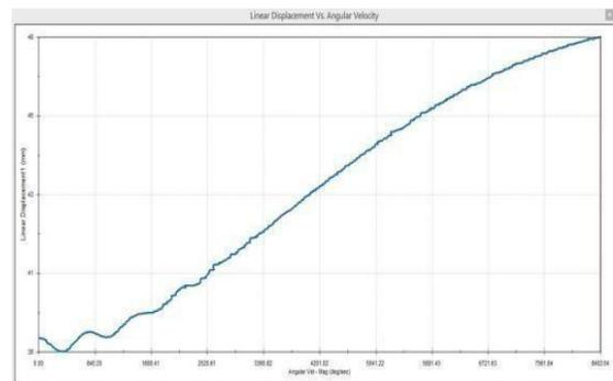
Figure 2. Graph between Angular Speed of Turbine & Displacement Covered By Masses.
